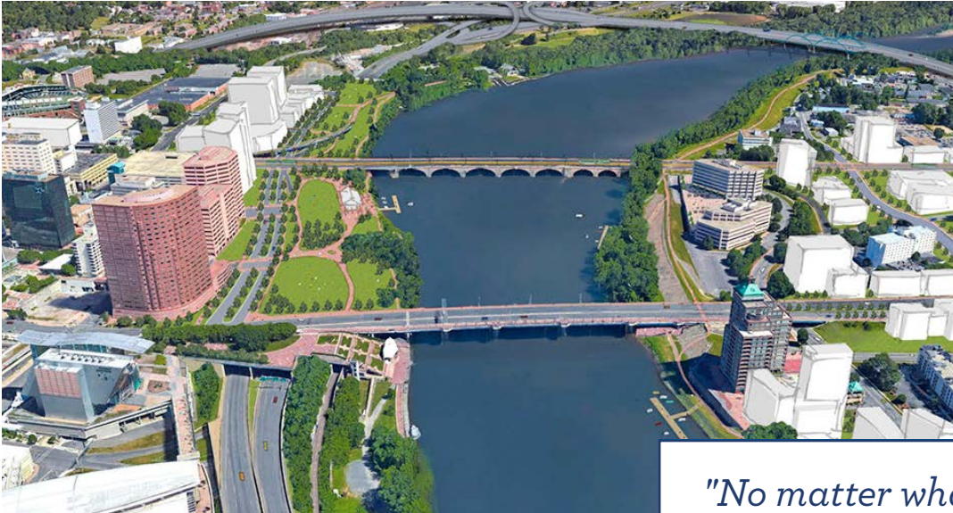
View north of downtown Hartford and East Hartford reveals the Bulkeley Bridge with reduced traffic and congestion, as well as a lowered and capped I-91 along the Connecticut River. As illustrated here in Concept 4, I-84 is relocated slightly north. Read the full description of all concepts starting on page two.
